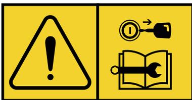
Turn off and remove key before repairing or servicing the machine.
